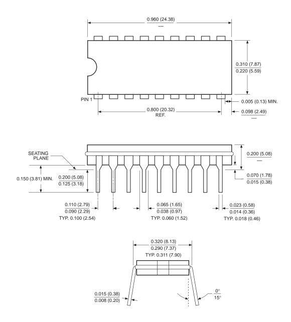
18-LEAD HERMETIC DUAL IN-LINE PACKAGE TYPE D
